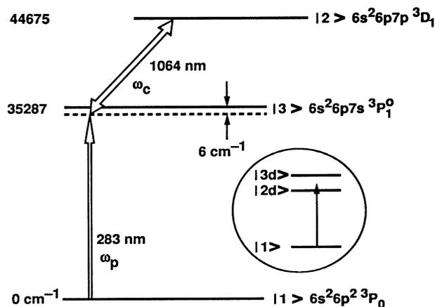
FIG. 1. Energy-level diagram of neutral Pb. Inset: Dressed-state picture.
