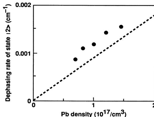
FIG. 5. State  $|2\rangle$  dephasing rate  $\gamma_{21}$  vs Pb density. The data points are obtained by curve fitting to measured transmission profiles. The dashed curve is calculated.
