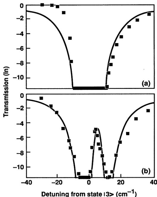
FIG. 4. Transmission vs probe laser detuning at 18 torr ( $N=1.2 \times 10^{17}$  atoms/cm<sup>3</sup>) for (a)  $\Omega_{23}=0$  and (b)  $\Omega_{23}=10.1$  cm<sup>-1</sup>. The solid curve is the fitted transmission spectrum.
