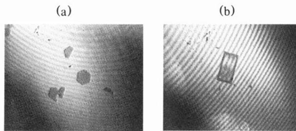
FIG. 1. Seeds of small growing ice crystals. (a) Hexagonal, basal orientation; surrounded by others of random orientation. (b) Rectangular, prism orientation.
