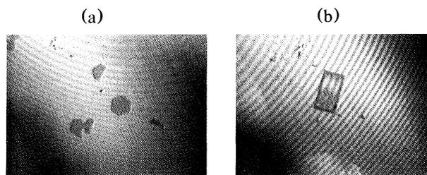
FIG. 1. Seeds of small growing ice crystals. (a) Hexagonal, basal orientation; surrounded by others of random orientation. (b) Rectangular, prism orientation.
