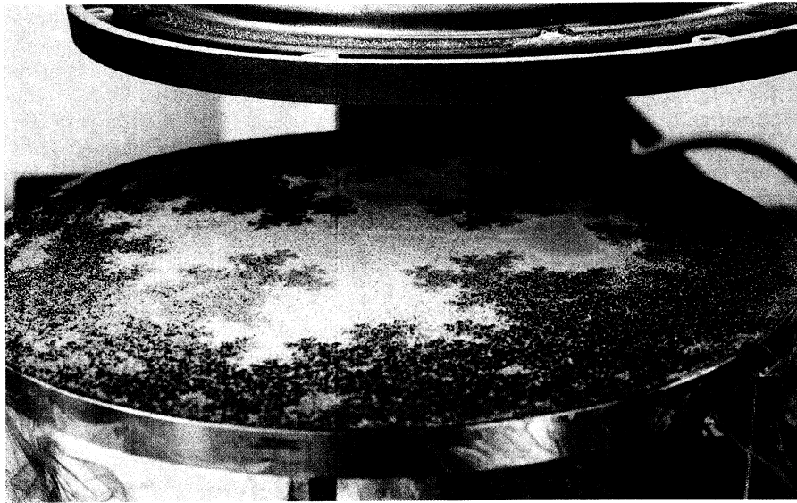
FIG. 2. Still photograph of a localized vibration (exposure time 1 s). In the vibrating region the light of the grazing laser is strongly scattered.
