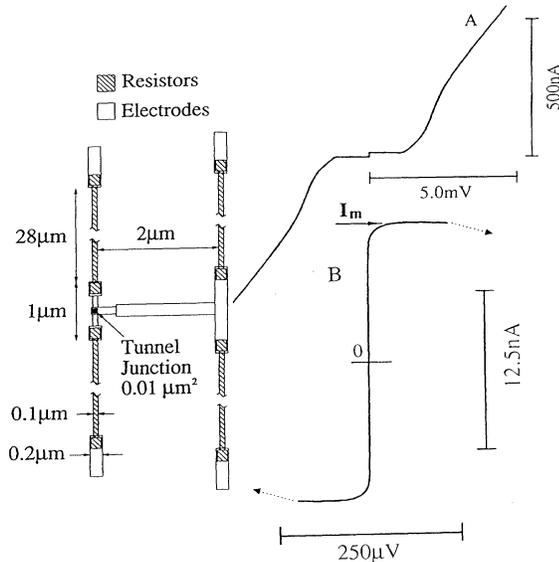
FIG. 1. The general shape of the dc  $I$ - $V$  curve of the junction (curve  $A$ ), and a blowup of its central part (curve  $B$ ) showing the current  $I_m$  where the  $I$ - $V$  curve jumps to the quasiparticle branch. Inset: The layout of our junction-plus-resistors circuit and the four-point dc measurement scheme.
