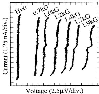
FIG. 2. The effect of the magnetic field on the dc  $I$ - $V$  curve at temperature  $T=70$  mK. The curves are offset along the  $V$  axis for clarity.
