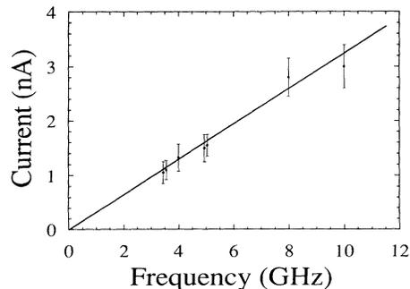
FIG. 4. The dc current  $I$ , which is the half-distance between the microwave-induced peaks of  $dV/dI$ , plotted as a function of the applied frequency  $f$ . Points show experimental data, while the line corresponds to the theoretical prediction  $I=2ef$ .
