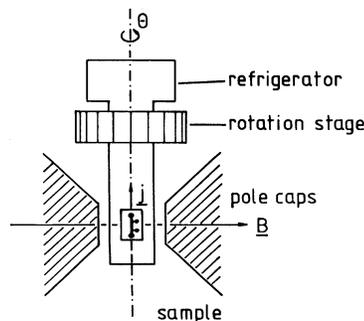
FIG. 1. Schematic of the setup used for the  $j_c(B, T, \Theta)$  measurements defining the angle  $\Theta$  between the magnetic-field direction and the  $c$  axis of the film.  $\Theta = 0$  corresponds to the  $B \parallel c$  direction.
