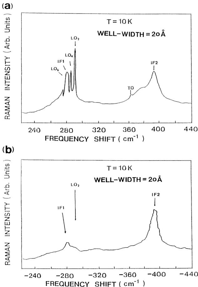
FIG. 1. (a) Stokes and (b) anti-Stokes Raman spectra of a GaAs/AlAs MQW with a 2-nm well width measured at 10 K with a train of 3-ps-long, 1.9-eV probe pulses which have been delayed by 1.5 ps relative to a train of 2.1-eV excitation pulses.
