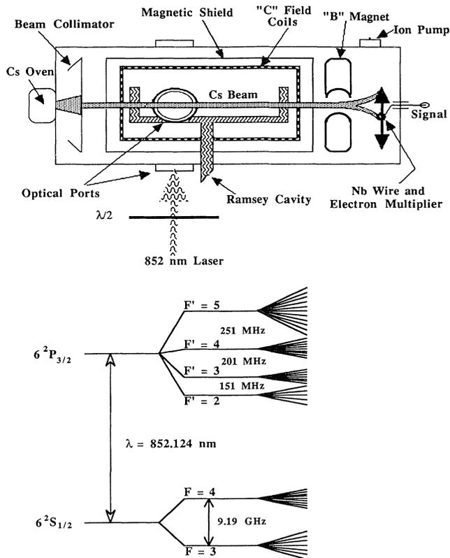
FIG. 1. Modified Cs atomic-clock tube and relevant Cs energy levels. The lifting of the degeneracy of each hyperfine level is shown as a function of a small magnetic field that was applied by the C-field Helmholtz coils.
