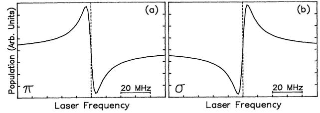
FIG. 3. Calculated population in the plus beam as a function of increasing laser frequency near the cycling transition for (a)  $\pi$  and (b)  $\sigma$  polarization, with a magnetic field of  $60 \text{ mG}$  and laser power of  $0.3 \text{ mW/cm}^2$ . The calculated  $\pi$ -polarization line shape was scaled by  $\sim 5 \times 10^3$  relative to the  $\sigma$ -polarization line shape.
