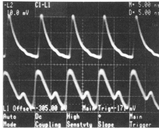
FIG. 4. The photovoltage (upper trace) in response to the *Q*-switched mode-locked laser pulses (lower trace) which have a width of 100 ps and a separation of 10 ns. The *Q*-switched envelope is 300 ns. The time resolution of the oscilloscope is 2 ns. The horizontal axis is 5 ns per division, and the vertical axis for the photovoltage is 10 mV per division.
