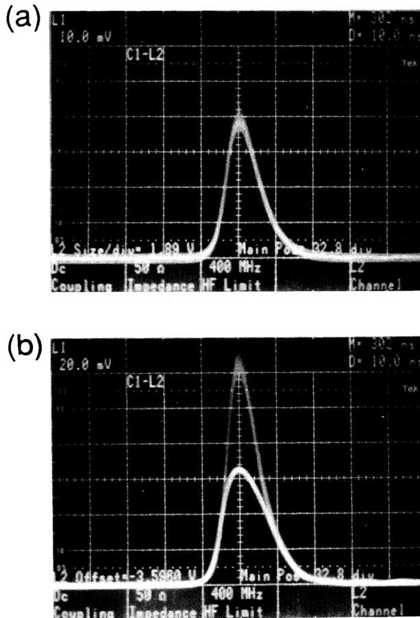
FIG. 2. The photovoltage signal (lower traces) generated by a 300-ns laser pulse (upper traces) which is monitored by a Si  $p$ - $i$ - $n$  detector. (a) When the laser intensity is low, the photovoltage signal follows linearly and coincides with the laser pulse signal. (b) When the laser intensity becomes high, the photovoltage saturates. The horizontal axis is 302 ns per division. The vertical axis is 10 and 20 mV per division in (a) and (b), respectively.
