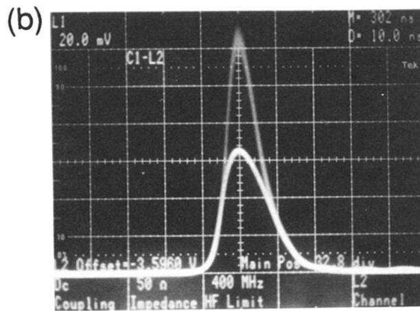
FIG. 2. The photovoltage signal (lower traces) generated by a 300-ns laser pulse (upper traces) which is monitored by a Si *p-i-n* detector. (a) When the laser intensity is low, the photovoltage signal follows linearly and coincides with the laser pulse signal. (b) When the laser intensity becomes high, the photovoltage saturates. The horizontal axis is 302 ns per division. The vertical axis is 10 and 20 mV per division in (a) and (b), respectively.
