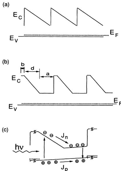
FIG. 1. The energy-band diagrams of the graded structures. (a) The sawtooth structure used in Ref. [1]. The present structure (b) in thermal equilibrium, and (c) under illumination.  $E_C$  is the conduction band edge, and  $E_V$  is the valence band edge.
