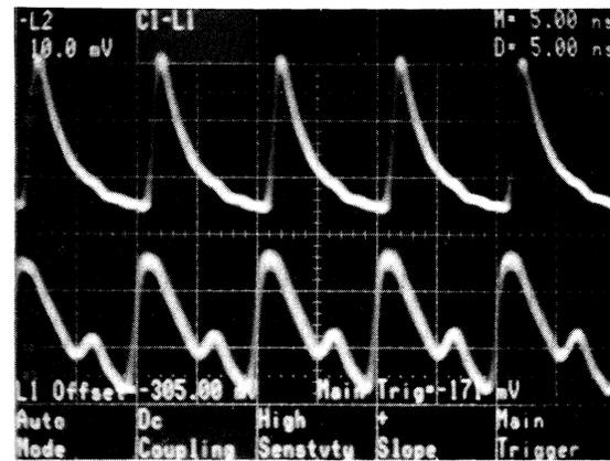
FIG. 4. The photovoltage (upper trace) in response to the  $Q$ -switched mode-locked laser pulses (lower trace) which have a width of 100 ps and a separation of 10 ns. The  $Q$ -switched envelope is 300 ns. The time resolution of the oscilloscope is 2 ns. The horizontal axis is 5 ns per division, and the vertical axis for the photovoltage is 10 mV per division.
