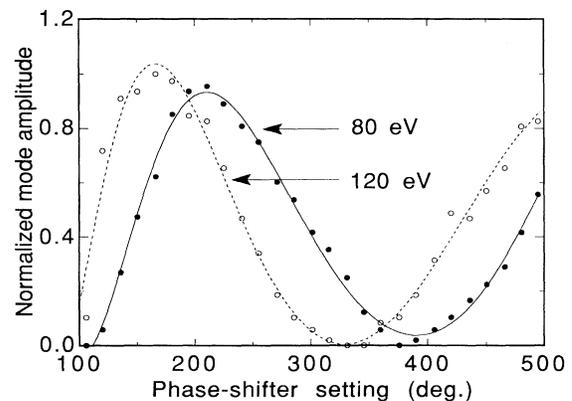
FIG. 6. Normalized mode amplitude vs the phase-shifter setting for two different values of ion-beam energy.
