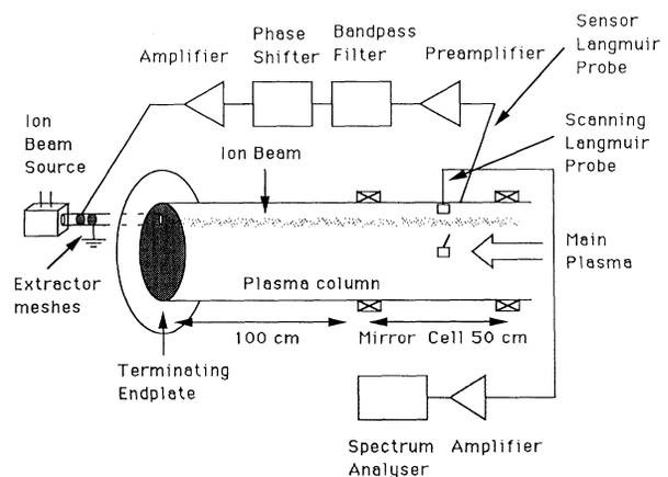
FIG. 1. Schematic of the experimental setup used for the feedback suppression of plasma instabilities via a modulated ion beam. The ion-beam source (IBS) is the remote suppressor and a Langmuir probe from a side port in the mirror cell is the sensor.
