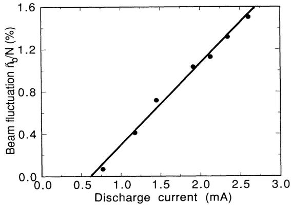
FIG. 4. Ion-beam fluctuation levels measured via a lock-in amplifier at 80 kHz for various values of the discharge current. The ion-beam density at 100% modulation is expressed as a percentage of the plasma density.
