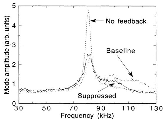
FIG. 3. Spectrum for the three cases of uncontrolled mode amplitude, suppressed mode amplitude, and the "noise" level taken with the mirror off.
