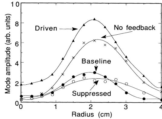
FIG. 5. A radial scan of the mode amplitudes for the four cases of maximum excitation, no feedback, maximum suppression, and "noise-level" base line, taken with the mirror off.
