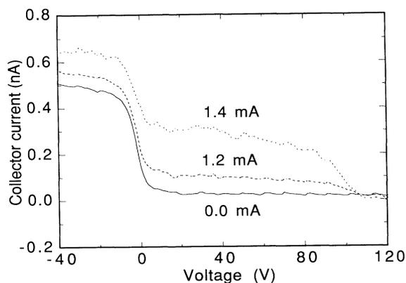
FIG. 2. Current-voltage characteristics of a gridded ion energy analyzer for three different values of discharge current. The extracted ion beam has energy of  $\sim 105$  eV and energy spread of  $\sim 20$  eV.
