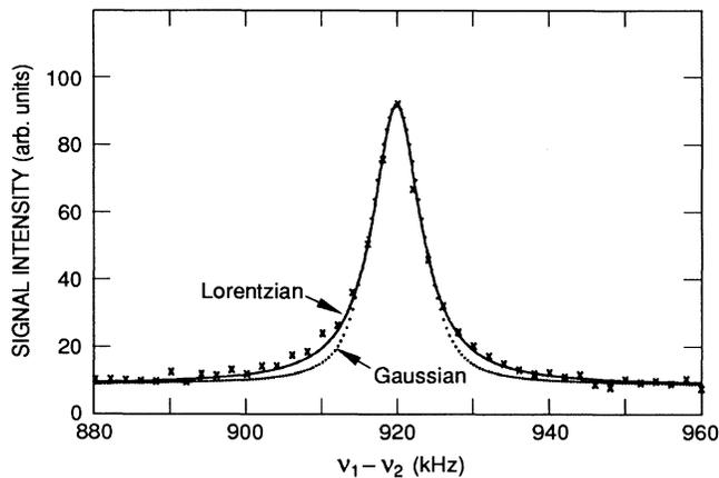
FIG. 2. FWM spectrum of the  $|\pm \frac{1}{2}\rangle \leftrightarrow |\pm \frac{3}{2}\rangle$  hyperfine transition. Experimental condition: same as Fig. 1 except  $t_p = 1.0$  ms. The solid curve is the calculated spectrum obtained using a Lorentzian line shape with  $\nu_0 = 919.8$  kHz and FWHM = 5.8 kHz. The dotted curve is that obtained using a Gaussian line shape with the same parameters.
