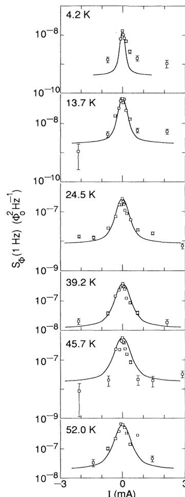
FIG. 3. Noise power  $S_\phi(1 \text{ Hz})$  vs current in transformer for six temperatures. The points are experimental data, from which the least noise measured at each temperature has been subtracted to remove background. The curves are the sum of predictions of Eq. (3) for each of the segments of the transformer. The central peak is due to input coil and the shoulders to pickup loop.
