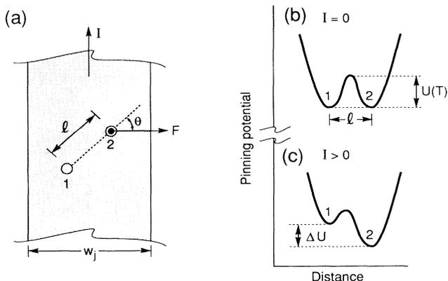
FIG. 4. (a) Schematic of single hopping process in line of width  $w_j$ . Current  $I$  exerts force  $F$  on the vortex which hops a distance  $l$  between pinning sites 1 and 2. The scale of  $l$  exaggerated. (b) Schematic pinning potential for  $I=0$ ; (c) for  $I>0$ .
