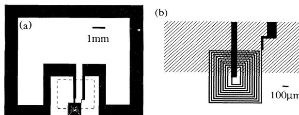
FIG. 1. YBCO flux transformer. (a) Pickup loop formed by wide lines, input coil centered on bottom edge, insulating  $\text{SrTiO}_3$  layer indicated by dashed box. (b) Enlargement of input coil: The shaded region is  $\text{SrTiO}_3$  and the vertical strip connected to the center of the coil is the cross under.
