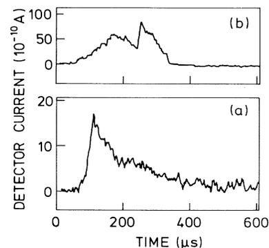
FIG. 1. Current pulse vs time from Si cleaved in vacuum received on (a) the Si detector and (b) the InSb detector.
