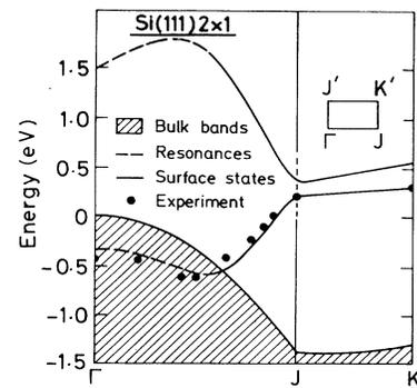
FIG. 4. Calculated (Ref. 12) dispersion of surface states for the optimized Pandey model. Experimental points (Ref. 15) have been shifted by 0.3 eV to match theory. Hatched area, bulk bands. Dashed lines, surface resonances. Solid lines, surface states. Inset: The two-dimensional Brillouin zone.
