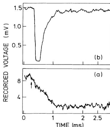
FIG. 2. Voltage detected by Si detectors from vacuum-cleaved Si using (a) a high-impedance input and (b) a shunt resistor across the input. In (b) a particularly large signal was obtained, which saturated the detector. In (a) the signal detection mode (the most sensitive) results in a changing base line while light is being received and a very slow recovery thereafter. The trigger time is shown with an arrow.
