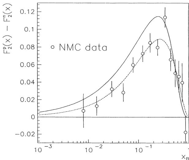
FIG. 1. Preliminary NMC data for the GSR for  $p_{\text{lab}}=280$  GeV and  $Q^2=4$  GeV<sup>2</sup>. The dashed line is a fit to the data using the parametrization given in the text and the solid line is from the global parametrization of MRS B.
