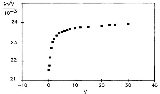
FIG. 3. The dependence of  $\lambda V^{1/2}$  on the growth velocity.
