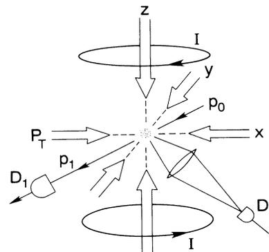
FIG. 1. Diagram of Zeeman-shift spontaneous-force optical trap (ZOT).
