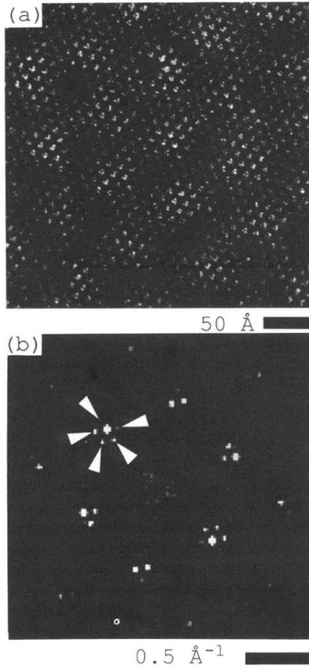
FIG. 2. (a) STM image of 1T-TaS<sub>2</sub> obtained at  $T=295$  K in the NC phase. (b) Fourier transform of (a). Satellite spots near hexagonally arranged CDW peaks are clearly evident; arrows identify five such spots. Different satellite spots have different intensities, consistent with theoretical predictions.
