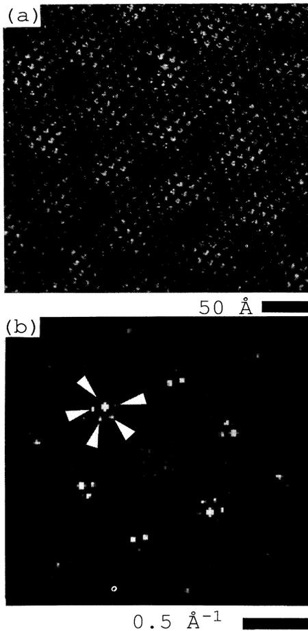
FIG. 2. (a) STM image of  $1T\text{-TaS}_2$  obtained at  $T=295$  K in the NC phase. (b) Fourier transform of (a). Satellite spots near hexagonally arranged CDW peaks are clearly evident; arrows identify five such spots. Different satellite spots have different intensities, consistent with theoretical predictions.
