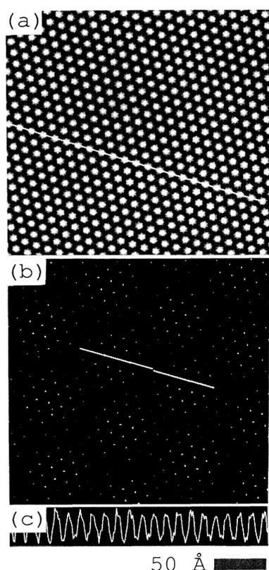
FIG. 1. (a) Computer-generated model image of  $1T\text{-TaS}_2$  at room temperature illustrating interference between atomic lattice and CDW. (b) Same image as (a) with gray scale adjusted to emphasize interference "domains." Computer-drawn lines pass through maxima in adjacent domains to show one-atomic-lattice-constant phase slip. (c) Intensity line scan through (a) demonstrating apparent CDW amplitude modulation.
