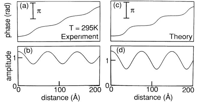
FIG. 3. (a) Real-space phase variation and (b) amplitude modulation  $A/A_{\text{avg}}$  of the CDW in  $1T\text{-TaS}_2$  in the NC phase reconstructed from the Fourier coefficients and wave vectors extracted from the Fourier transform of Fig. 2(a). (c) Real-space phase variation and (d) amplitude modulation  $A/A_{\text{avg}}$  of the CDW predicted by the Nakanishi and Shiba theory.
