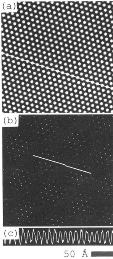
FIG. 1. (a) Computer-generated model image of  $1T\text{-TaS}_2$  at room temperature illustrating interference between atomic lattice and CDW. (b) Same image as (a) with gray scale adjusted to emphasize interference "domains." Computer-drawn lines pass through maxima in adjacent domains to show one-atomic-lattice-constant phase slip. (c) Intensity line scan through (a) demonstrating apparent CDW amplitude modulation.
