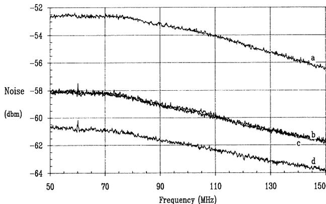
FIG. 2. Amplitude fluctuation spectra of the laser field (traces *b* and *c*) and LED (trace *a*) for identical detector currents of 8.6 mA. The laser is either coupled to a different detector (trace *b*) or to the same detector (trace *c*) as the LED. Trace *d* is the amplitude noise at a higher pump level, and the corresponding detector current was 11.3 mA. In this case the shot-noise level was also set equal to trace *a*. The thermal background noise was subtracted from all of the traces.
