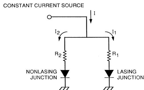
FIG. 3. A model for current division into a lasing junction and a nonlasing junction.
