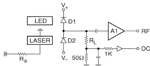
FIG. 1. The principal elements of the experimental apparatus that were inside the cryostat. The power spectrum of the amplified photocurrent is displayed on a spectrum analyzer (not shown), and the average detector current is monitored at the output labeled dc.
