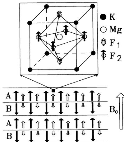
FIG. 1. Two-sublattice ferromagnet with domains for the external field  $B_0$  parallel to [100] at negative temperature. The spins 1 and 2 are identified in the elementary cell.
