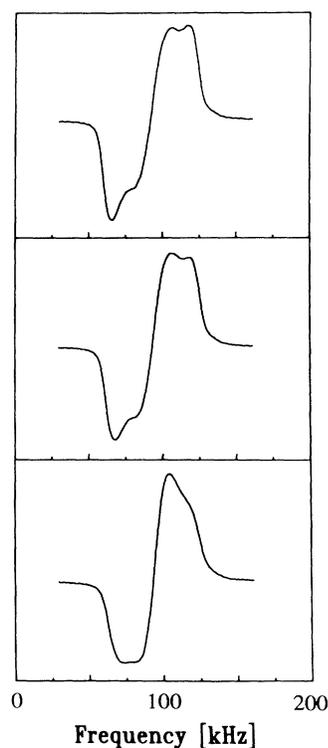
FIG. 4.  $^{19}\text{F}$  absorption signals of orientation [100] at negative temperature. Upper and middle signals: ferromagnetic phase with domains; lower signal: paramagnetic phase. The origin of frequencies is arbitrary.
