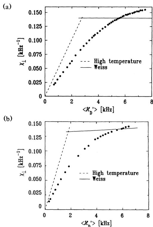
FIG. 3. Transverse susceptibility  $\chi_\perp$  as a function of the dipolar energy  $\langle \mathcal{H}^d \rangle$ . (a) Orientation [111], negative temperature; (b) orientation [100], negative temperature.
