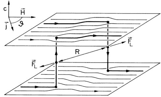
FIG. 3. Nucleation process in the vortex liquid. The vanishing interlayer shear has led to the melting of the elastic string present in the vortex lattice. After relaxation, a pair of edge dislocations (magnetic monopoles) appears in each plane with a logarithmic interaction between the two monopoles constituting each pair.
