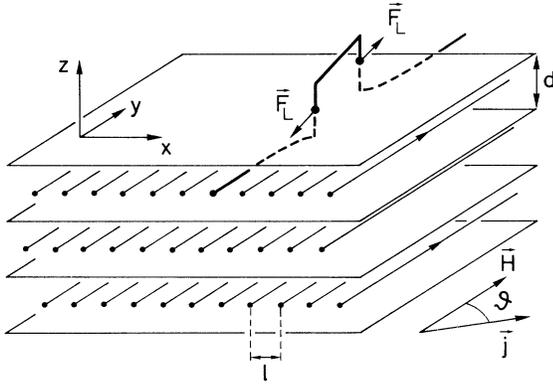
FIG. 1. Vortex structure for large magnetic fields  $H \geq H_d$  in a strongly layered superconductor. At high enough temperatures the vortex lattice melts and the interlayer shear modulus vanishes, resulting in a smectic vortex state as illustrated (drawing not to scale).
