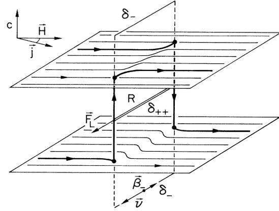
FIG. 2. Nucleation process in the vortex lattice. The moving pancake vortices (vertical segments of the loop) generate a string of three dislocations  $\mathbf{v}_-$ ,  $\mathbf{v}_{++}$ , and  $\mathbf{v}_-$  along their path with the total topological charge zero (drawing not to scale).
