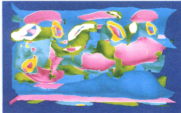
FIG. 8. Same calculation as in Fig. 7. Cross section of the longitudinal vortices: yellow, streamwise vorticity w_x = +0.8U_0/H ; white, w_x = -0.8U_0/H .
