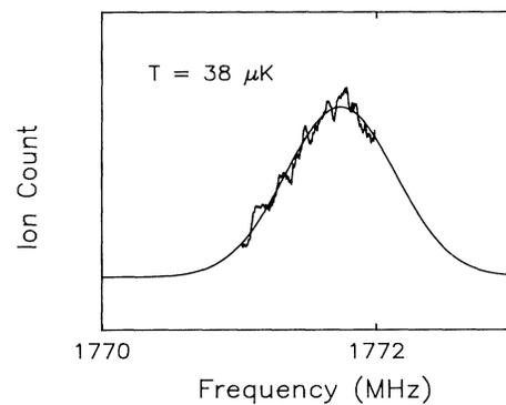
FIG. 4. A measurement of the transverse velocity distribution of the atoms in the atomic fountain. The temperature is slightly higher than what is usually achievable with polarization gradient molasses cooling because of the small amount of heating due to optical pumping.
