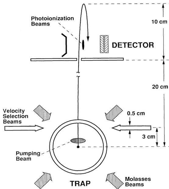
FIG. 2. A schematic diagram of the velocity-selection apparatus. The pumping beam and the photoionization beams are propagating normal to the paper. Not shown are the other set of molasses beams and the slowing beam used to load the magneto-optic trap.
