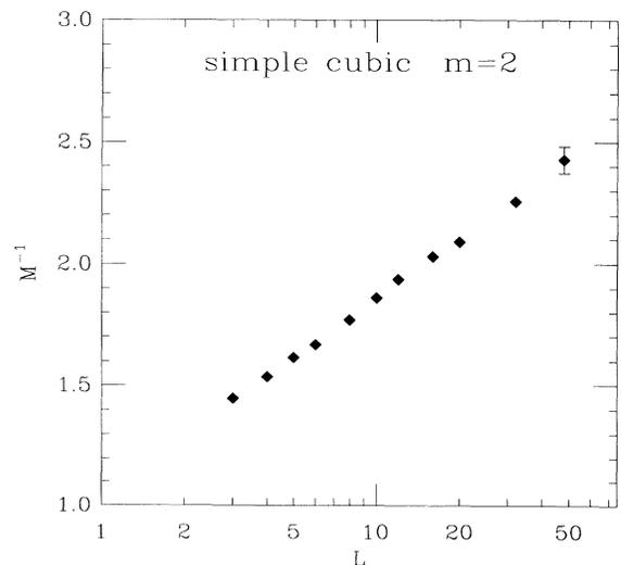
FIG. 1. Inverse of the average magnetization (as defined in the text),  $1/M$ , vs lattice size,  $L$ , for  $L \times L \times L$  simple cubic lattices, for the random-anisotropy model with  $m=2$  and  $D/J = \infty$ . The  $L$  axis is scaled logarithmically. The error bars for  $L=48$  show 1 standard deviation. The error bars for smaller  $L$  would be about the same size as the plotting symbols.
