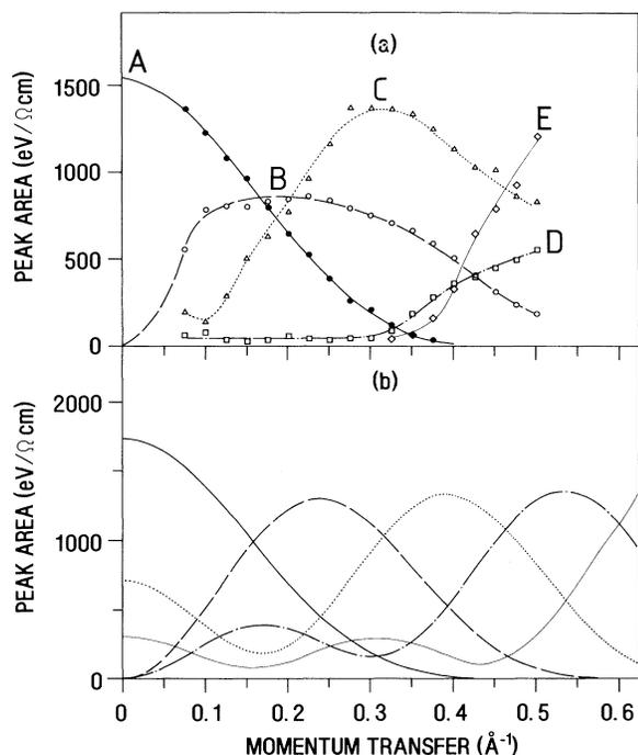
FIG. 3. Intensity of the various lines detected in the optical conductivity as a function of momentum transfer  $q$  parallel to the  $b$  axis. (a) Experimental data and (b) theoretical values.
