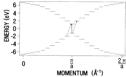
FIG. 2. Quasi band structure for the  $\pi$  electrons in  $\beta$ -carotene. The vertical 1-1\* transition and the nonvertical 2-1\* and 1-2\* transitions are shown.
