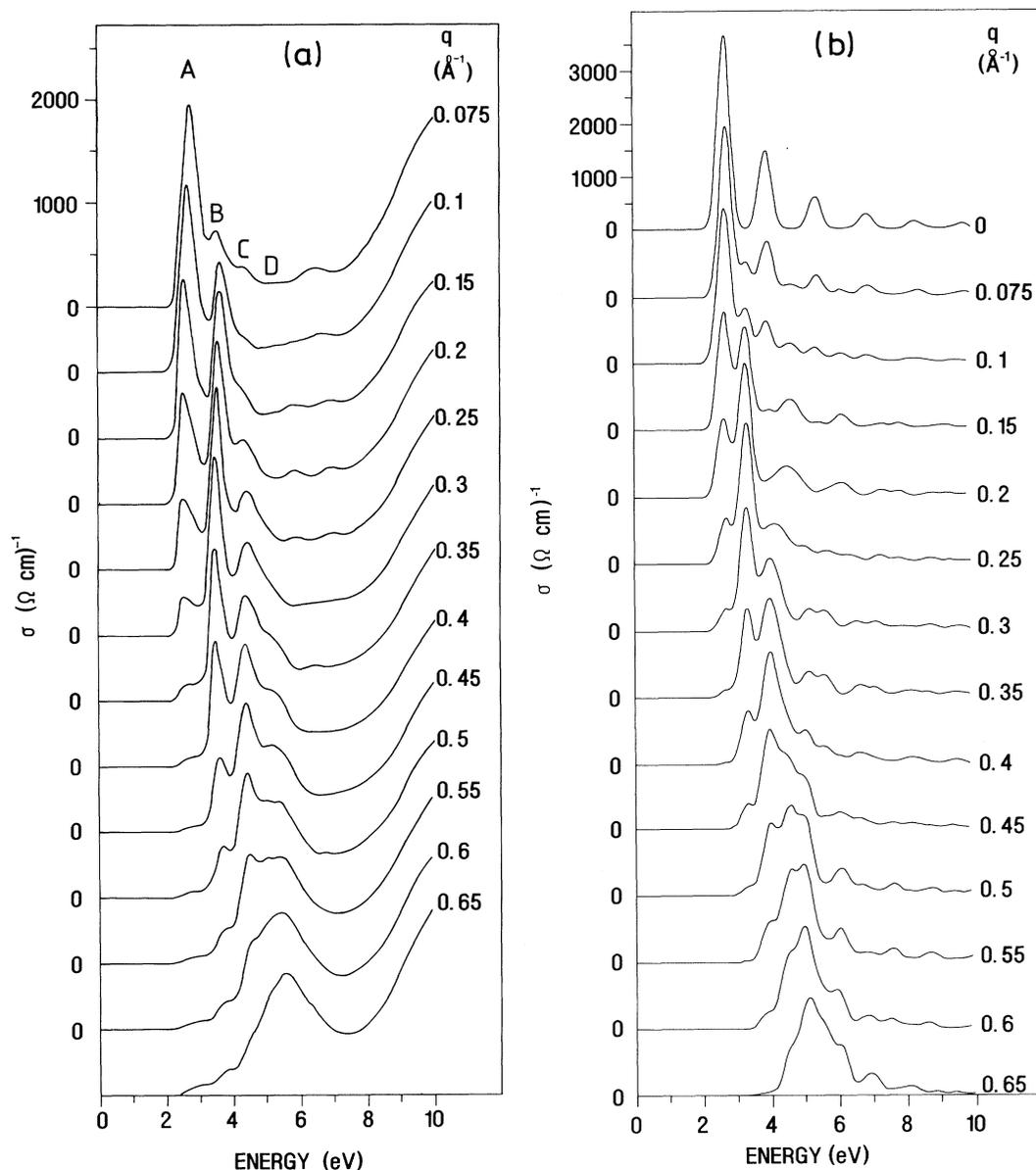
FIG. 1. Momentum-dependent optical conductivity of  $\beta$ -carotene. (a) Experimental data derived from EELS measurements. (b) Theoretical data.
