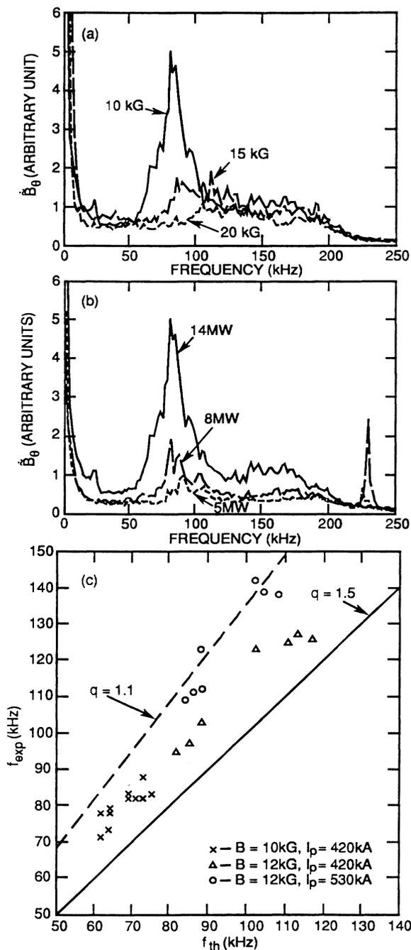
FIG. 1. (a) Frequency spectrum of Mirnov-coil signal from plasmas with  $\langle \beta \rangle \sim 1\%$  at various magnetic fields. (b) Variation of frequency spectrum with neutral-beam power. (c) Comparison of experimentally measured frequencies with theoretically calculated TAE frequencies.
