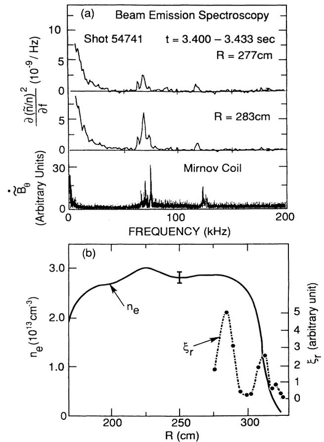
FIG. 2. (a) Comparison of fluctuation spectra from beam-emission-spectroscopy data and Mirnov-coil data. (b) Variation of inferred plasma radial displacement and electron-density profile.
