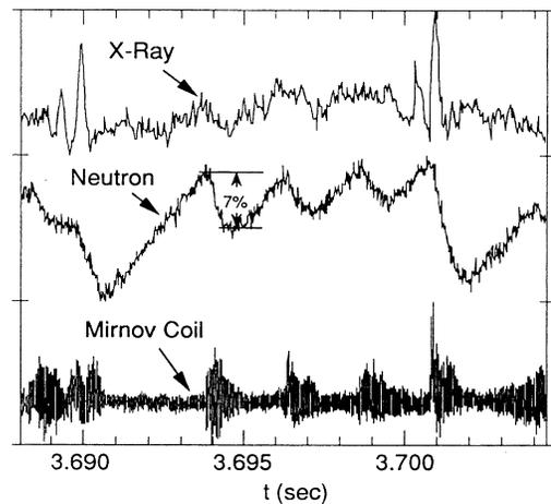
FIG. 4. Correlation between Mirnov-coil signal at  $\theta=0$  (bottom trace), total neutron-emission rate (middle trace), and soft-x-ray emission at  $r=4$  cm (top trace) from the plasma. The vertical scale is linear with zeros suppressed.
