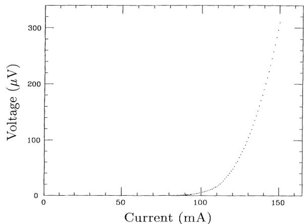
FIG. 4. Voltage-current characteristics of the bridge in Fig. 1(b) at 77 K.
