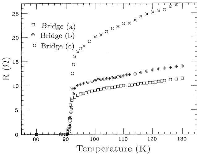
FIG. 2. Temperature dependence of the resistance of the three microbridges.
