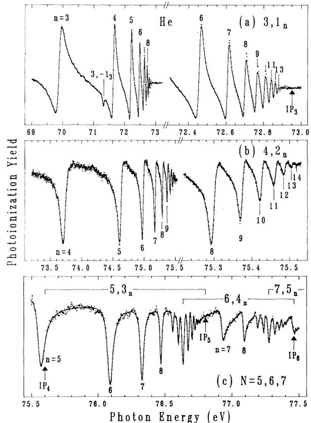
FIG. 2. Autoionizing states of He: (a) below the  $N=3$  threshold ( $IP_3$ ), (b) below the  $N=4$  threshold ( $IP_4$ ), and (c) below the  $N=5$  and 6 thresholds ( $IP_5$ ,  $IP_6$ ). The high- $n$  regions are shown magnified on the right-hand sides in (a) and (b). Note the overlapping of series in (c).
