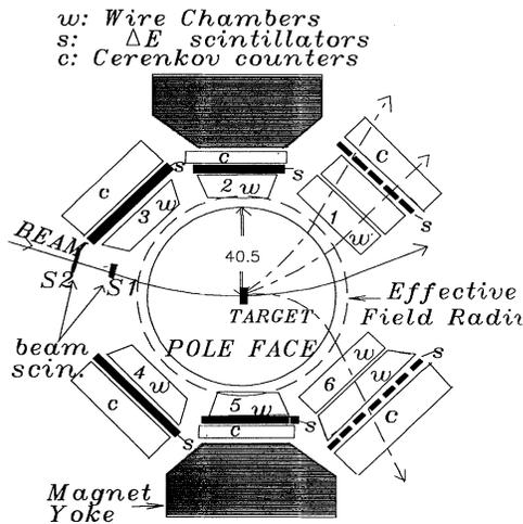
FIG. 1. Layout of the CALLIOPE spectrometer. The dashed lines represent scattered particles.
