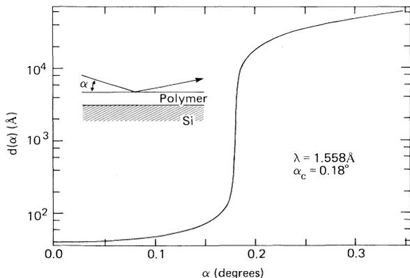
FIG. 1. Variation of the incident x-ray penetration depth for polyimide as a function of the angle of incidence. Below the critical angle  $\alpha_c$ , the penetration depth ranges between 50 and  $100 \text{ \AA}$ , while above  $\alpha_c$ , it is nearly equal to the attenuation length times  $\sin\alpha$ .
