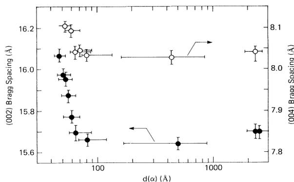
FIG. 3. Bragg spacings corresponding to the (002) (●) and (004) (○) reflections for PMDA-ODA as a function of incident-beam penetration depth. The vertical error bars were determined from the standard deviation in the peak position of fitted profiles to the experimental data, whereas the horizontal error bars show the range of penetration depths for a given  $\alpha$  with a 1-mrad angular divergence.
