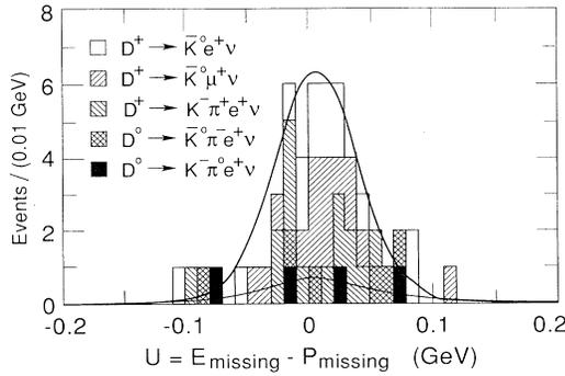
FIG. 2. The  $U$  distribution for semileptonic decays. The heavy and light curves are Monte Carlo predictions for the all-charged channels and the  $D^0 \rightarrow K^- \pi^0 e^+ \nu_e$  channel, respectively.
