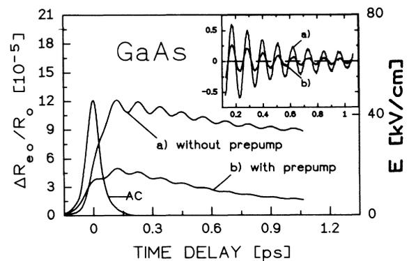
FIG. 2. Electro-optic signal changes at the GaAs surface at (a) an excitation density of approximately  $10^{18}$  cm $^{-3}$  and (b) with prepump excitation ( $> 10^{18}$  cm $^{-3}$ ) at a time delay of  $\Delta t = -10$  ps. Inset: Oscillatory signal part.
