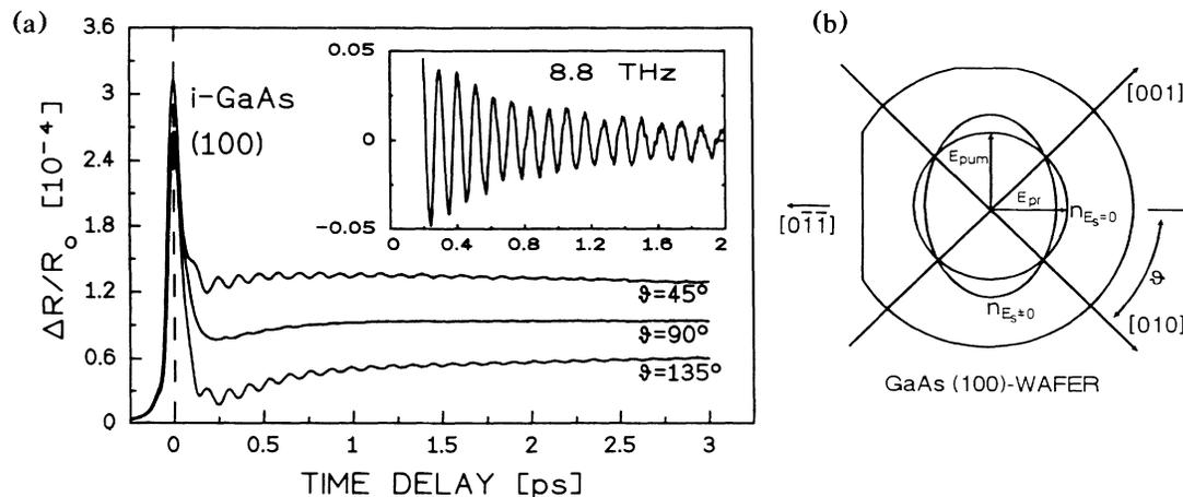
FIG. 1. (a) Time-resolved reflectivity changes of (100)-oriented intrinsic GaAs at an excitation density of  $N = 10^{18} \text{ cm}^{-3}$  for orthogonal polarization of pump and probe beam. (b) The parameter  $\vartheta$  is the angle between probe polarization and [010] crystal axis. Also shown is the projection of the index ellipsoid on the surface of a (100)-oriented wafer in the case of zero and nonzero applied field in the [100] direction, e.g., perpendicular to the surface.
