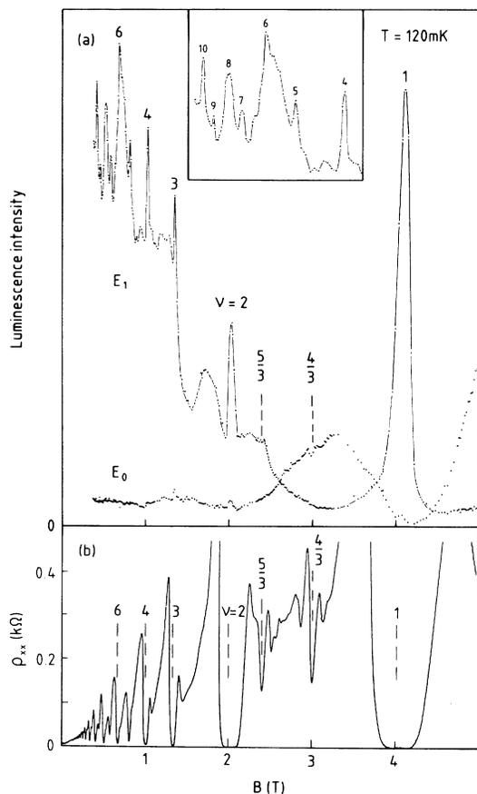
FIG. 2. (a) Intensities of the  $E_0$  and  $E_1$  luminescence lines at 120 mK as a function of magnetic field for  $\nu \geq 1$ . Inset: Region  $\nu=10$  to 4 on an expanded scale. (b) Simultaneous  $\rho_{xx}$  data.
