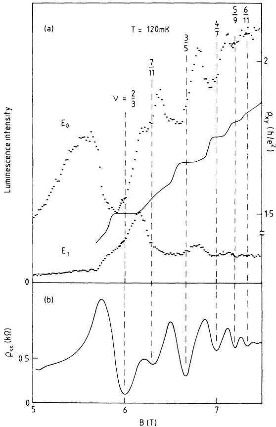
FIG. 3. (a) Intensities of the  $E_0$  and  $E_1$  luminescence lines at 120 mK for  $\nu < 1$ . (b) Simultaneous  $\rho_{xx}$  data. Also shown in (a) is a  $\rho_{xy}$  trace from a Hall bar sample at a similar temperature in the absence of laser illumination.
