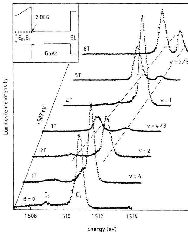
FIG. 1. Selected photoluminescence spectra at 120 mK in the field range  $B=0-6$  T. Inset: Sample structure (see text) and  $E_0, E_1$  energies.
