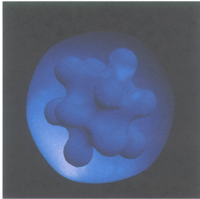
FIG. 5. Three-dimensional shape of the contact surface showing nonlinear bubble-spike structures for (n,m) = (6,3) .
