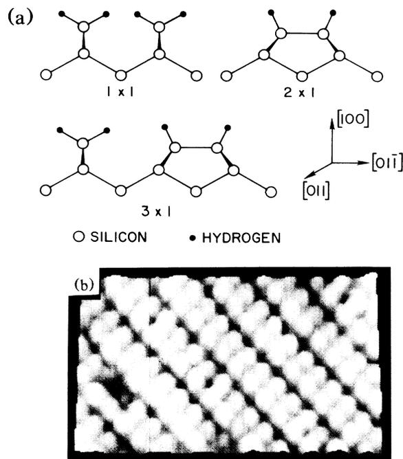
FIG. 1. (a) Schematic of the various possible hydrogenated structures present on the Si(100) surface. (b) Scanning-tunneling-microscopy (STM) topograph of the monohydride phase. The surface shown is  $59 \times 39$  Å and the image was recorded at a sample bias of +2.5 V.
