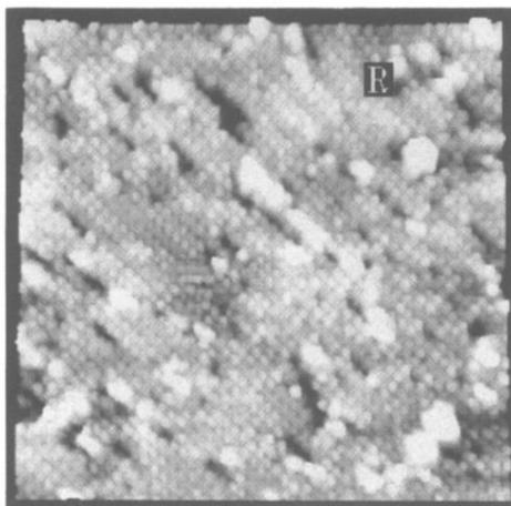
FIG. 3. STM topograph of the unoccupied states (+3 V) of the  $3\times 1$  surface following a RT exposure to atomic H. *R* denotes remnants of the  $3\times 1$  phase. The area shown is  $181\times 194$  Å.
