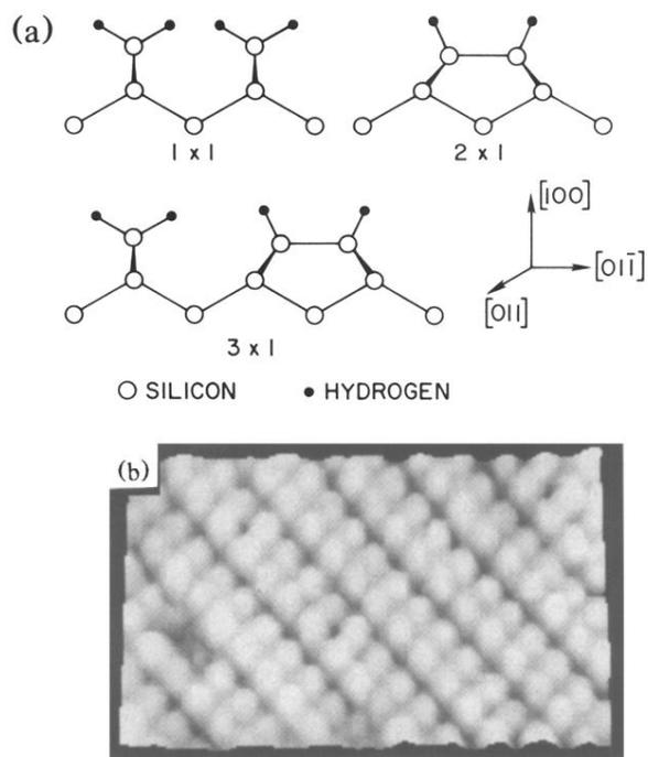
FIG. 1. (a) Schematic of the various possible hydrogenated structures present on the Si(100) surface. (b) Scanning-tunneling-microscopy (STM) topograph of the monohydride phase. The surface shown is  $59 \times 39 \text{ \AA}$  and the image was recorded at a sample bias of +2.5 V.
