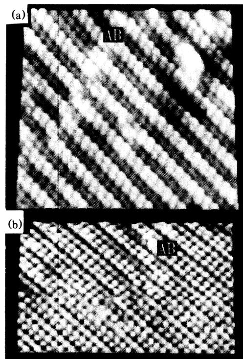
FIG. 2. (a) STM topograph of the unoccupied states (+2 V) on the 3 $\times$ 1 phase. The area shown is 104 $\times$ 107 Å. There is a slight uncorrected thermal drift in this image. (b) STM topograph of the occupied states (−2 V) on the 3 $\times$ 1 phase. The area shown is 108 $\times$ 75 Å. AB denotes the presence of 3 $\times$ 1 antiphase boundaries.
