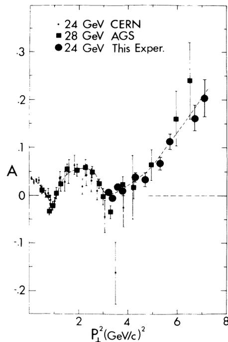
FIG. 2. The analyzing power  $A$  as a function of momentum transfer squared  $P_\perp^2$  for spin-polarized proton-proton elastic scattering at 24 GeV/ $c$ . The error bars include both the statistical and systematic errors. Other data at 28 (Ref. 4) and 24 GeV/ $c$  (Ref. 25) are also shown. The dashed curve is a hand-drawn curve to guide the eye.
