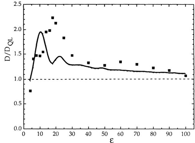
FIG. 2. Ratio of the diffusion coefficient to the quasilinear value shown as squares for the Hamiltonian (2) and as a solid curve for the randomly phased, two-step mapping (3).
