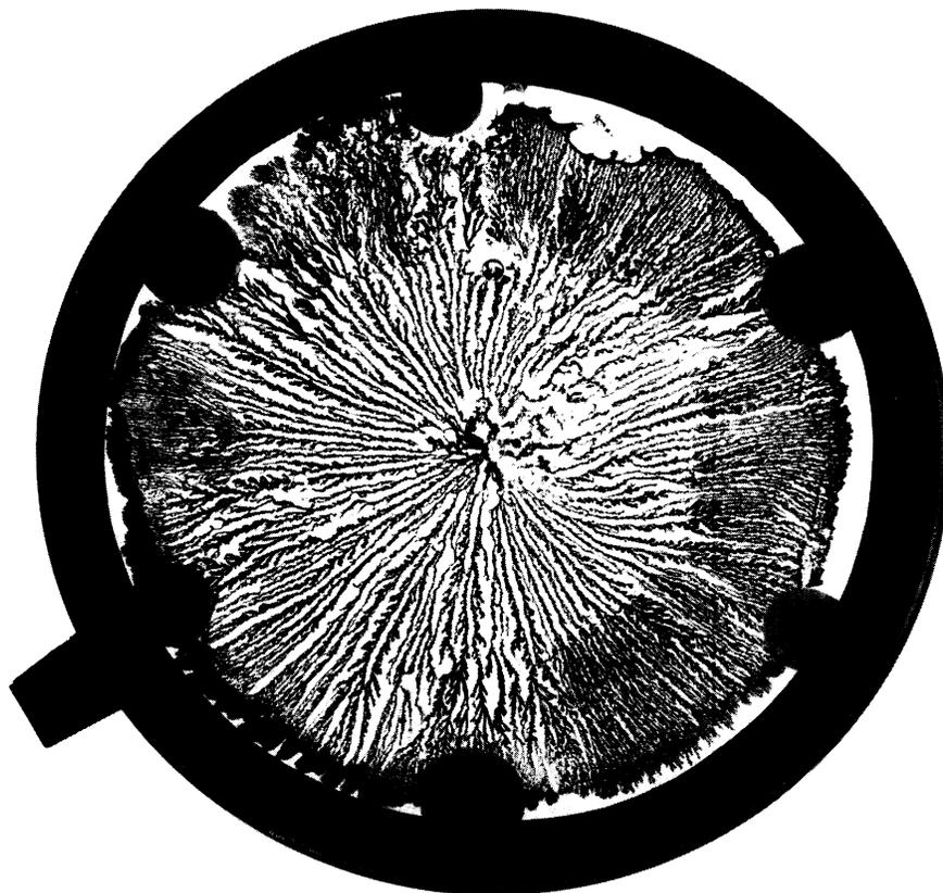
FIG. 1. A deposit within a thin cell of radius 3.0 cm, at an applied potential of 25 V from a  $0.05\text{-mol dm}^{-3}$   $\text{CuSO}_4$  solution. From 12 to 5 o'clock a distinct branching (Hecker) transition is observed at  $0.5L_A$ . From 4 to 9 o'clock the third transition mentioned in the text is evident at  $0.9L_A$ .
