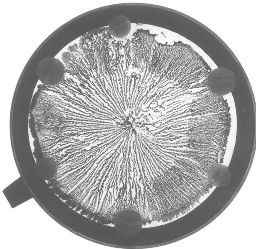
FIG. 1. A deposit within a thin cell of radius 3.0 cm, at an applied potential of 25 V from a  $0.05\text{-mol dm}^{-3}$   $\text{CuSO}_4$  solution. From 12 to 5 o'clock a distinct branching (Hecker) transition is observed at  $0.5L_A$ . From 4 to 9 o'clock the third transition mentioned in the text is evident at  $0.9L_A$ .
