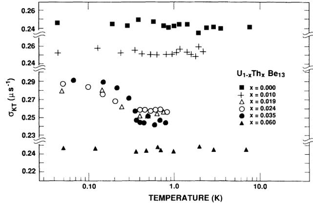
FIG. 1. Temperature dependence of the zero-field  $\mu$ SR rate  $\sigma_{KT}(T)$  for various Th concentrations  $x$  in  $U_{1-x}Th_xBe_{13}$ .
