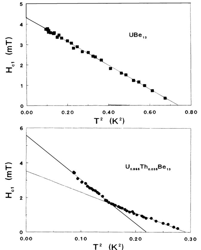
FIG. 2.  $H_{c1}(T)$  plotted vs  $T^2$  in  $U_{1-x}Th_xBe_{13}$  for  $x=0.0000$  (top) and  $x=0.0355$  (bottom). The lines are guides to the eye.
