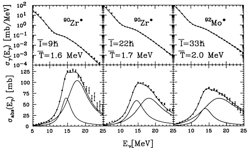
FIG. 2. Top row: measured and fitted  $\gamma$ -emission cross section  $\sigma_\gamma(E_\gamma)$ . Bottom row: solid curves, fitted absorption cross section  $\sigma_{\text{abs}}(E_\gamma)$  corresponding to the parameters given in Table I; data points, measured  $\sigma_\gamma(E_\gamma)$  divided by the calculated ratio  $\sigma_\gamma(E_\gamma)/\sigma_{\text{abs}}(E_\gamma)$ .
