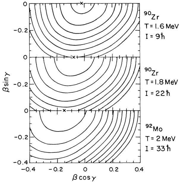
FIG. 1. Calculated potential-energy (free-energy) surfaces for the three cases of interest (Ref. 10). Contour lines are spaced every 1 MeV. Crosses indicate the locations of the minima, which lie along the oblate noncollective axis ( $\gamma = -180^\circ$ ). These surfaces demonstrate the expected nuclear shape change from spherical to oblate.
