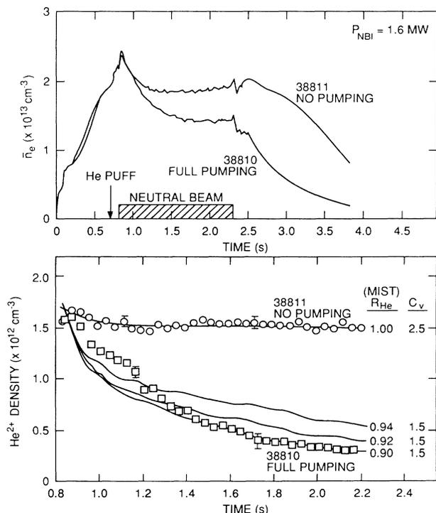
FIG. 1. Line-averaged electron density  $\bar{n}_e$  and  $\text{He}^{2+}$  density measured with CXE spectroscopy vs time during low-density plasma discharges after a short He puff at 0.7 s with and without ALT-II pumping and 1.6-MW NBI. Points:  $\text{He}^{2+}$  density data; solid lines: MIST transport calculations.
