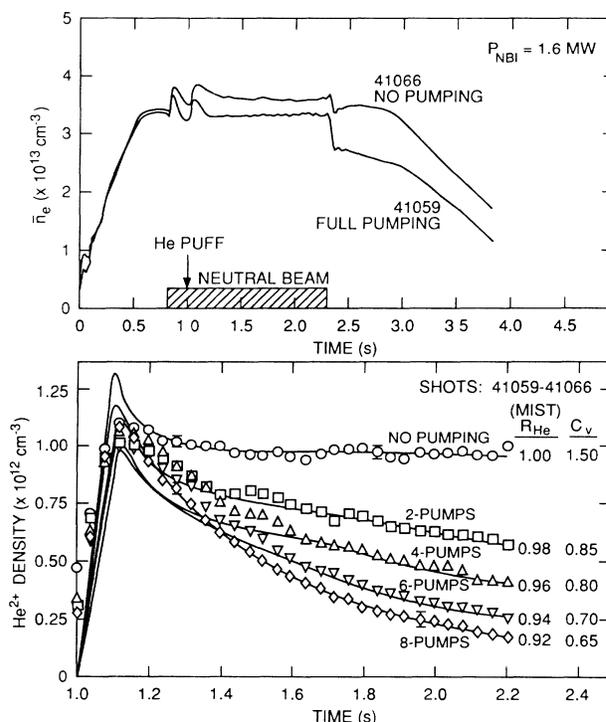
FIG. 2. Line-averaged electron density  $\bar{n}_e$  and  $\text{He}^{2+}$  density measured with CXE spectroscopy vs time during higher-density plasma discharges after a short He puff at 1.0 s with and without ALT-II pumping and 1.6-MW NBI. Points:  $\text{He}^{2+}$  density data; solid lines: MIST transport calculations.
