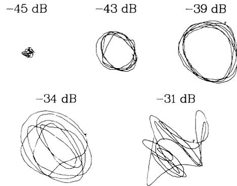
FIG. 2. Experimental phase portraits for various feedback levels.  $J/J_{th}=1.83$ ,  $\tau=1.07$  ns.
