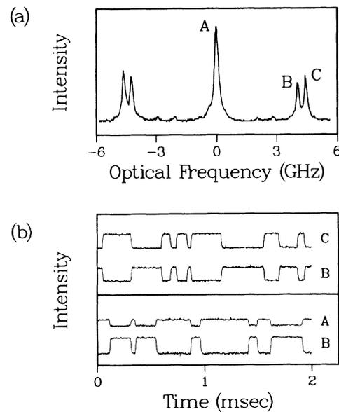
FIG. 4. (a) Time-averaged optical spectrum. The frequency of the solitary laser corresponds to 0 GHz. (b) Time dependence of peaks *B* and *C* (upper two traces) and *A* and *B*. Dotted lines indicate zero intensity level (common for two lower traces).  $J/J_{th} = 2.01$ ,  $\tau = 1.97$  ns,  $\kappa^2 = -37$  dB.
