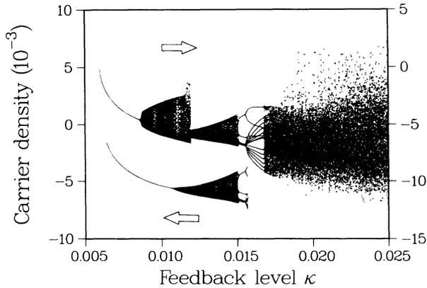
FIG. 1. Calculated bifurcation diagram for  $J/J_{th}=2.0$  and  $\tau=2$  ns. The upper part (right axis) is obtained for increasing  $\kappa$  and the lower part (left axis) is obtained for decreasing  $\kappa$ . The traces are separated vertically for clarity.
