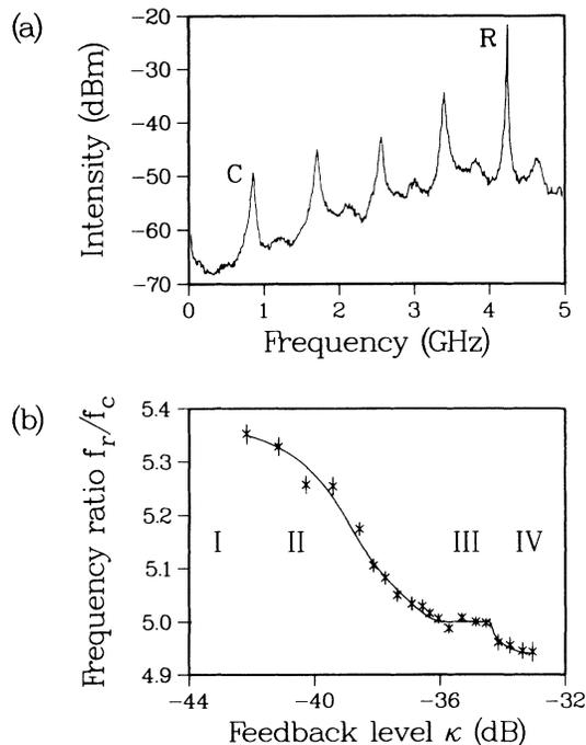
FIG. 3. (a) Measured intensity spectrum and (b) frequency ratio  $f_r/f_c$  vs feedback level with identification of regimes I (limit cycle), II (quasiperiodic), III (frequency locked), and IV (chaotic).  $J/J_{th} = 1.84$ ,  $\tau = 1.07$  ns.
