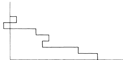
FIG. 1. Typical configuration showing displacement parallel to substrate as function of height above substrate.
