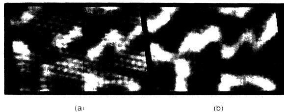
FIG. 1. Two images of the Au/Si(111) \sqrt{3} \times \sqrt{3} structure, taken concurrently with tip bias voltages (a) V_T = -1.9 V, (b) V_T = +0.2 V, and a tunneling current I_T = 2.7 nA.
