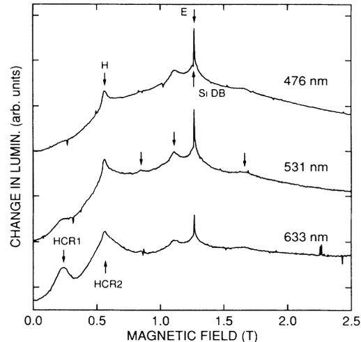
FIG. 2. ODMR spectra obtained at 35 GHz with  $\mathbf{B}$  along the [001] axis for three excitation wavelengths. Peaks are labeled according to the assignments described in the text.
