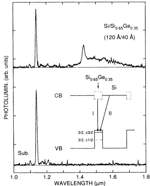
FIG. 1. Photoluminescence spectra of the front (superlattice) and back (substrate) surfaces obtained at 1.6 K with 633-nm excitation. Inset: Schematic representation of energy band structure as described in text. Type-I and -II recombination transitions are both shown due to the uncertainty in the location of the conduction-band (CB) minimum in the superlattice.
