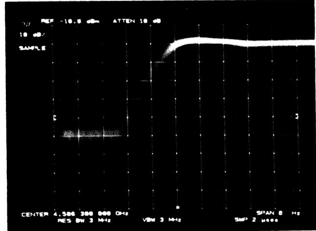
FIG. 4. The growth and decay of the intensity of Bragg scattering signal during the first 2- $\mu$ sec period.
