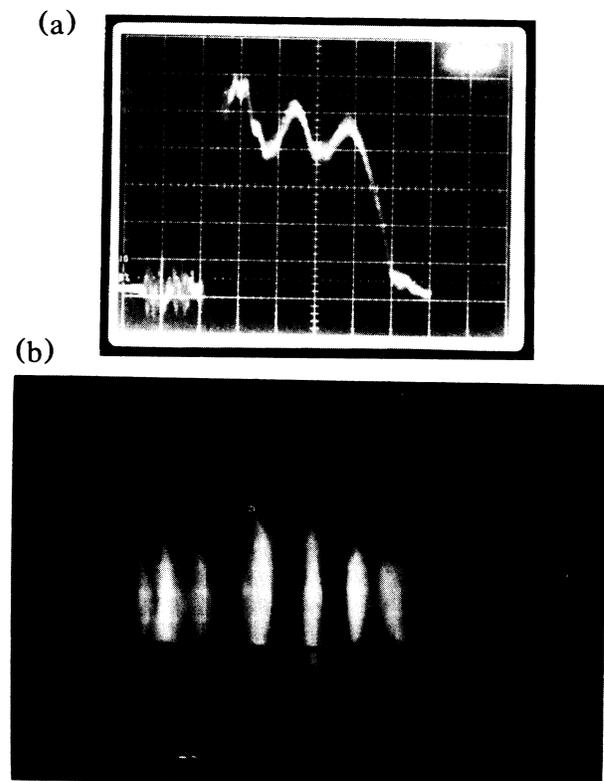
FIG. 1. (a) Envelope of a 1- $\mu$ sec microwave pulse. (b) A photo of plasma layers generated by two cross pulses having parallel polarization.
