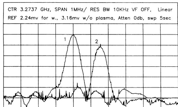
FIG. 3. Frequency spectra of two output pulses with same input. Curve 1 is the spectrum of the pulse passing through the chamber (at the pressure  $\sim 1$  atm) without plasma generation and curve 2 represents the spectrum of the pulse passing through a rapidly growing plasma generated inside the chamber (at the pressure  $\sim 2.3$  Torr).
