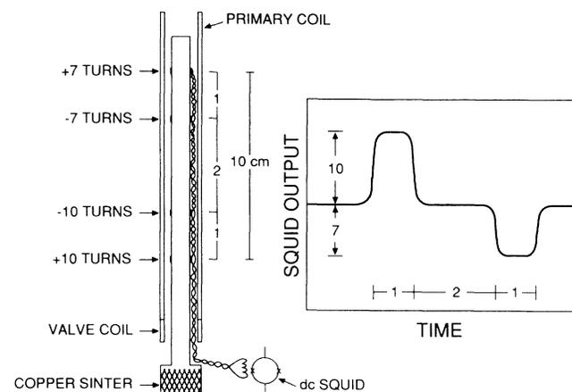
FIG. 1. The experimental cell. The four coils span a total length of 10.1 cm. Inset: The "nominal magnetization signature" generated by the simplest  $AB$  interface.
