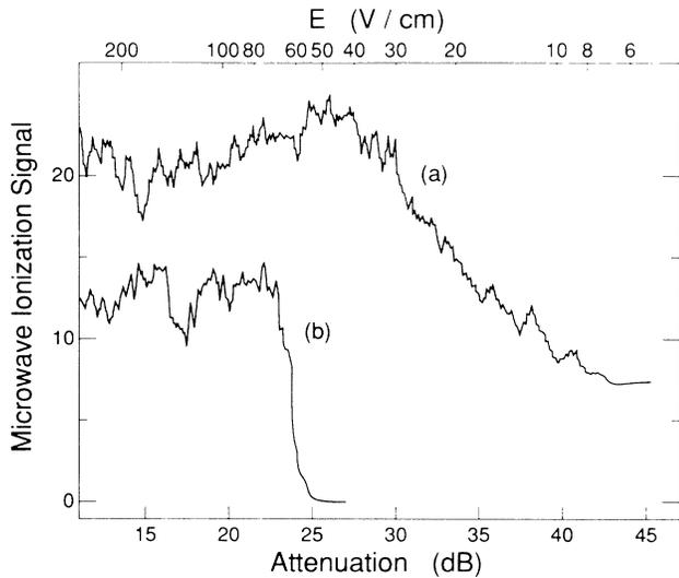
FIG. 1. Microwave ionization signals as a function of microwave attenuation when the Rydberg atoms are excited in the microwave field at the energy of the  $46d$  state; curve *a*, linearly polarized microwaves and curve *b*, circularly polarized microwaves. The two traces are offset vertically by eight units for clarity. For reference a microwave field scale is shown as well.
