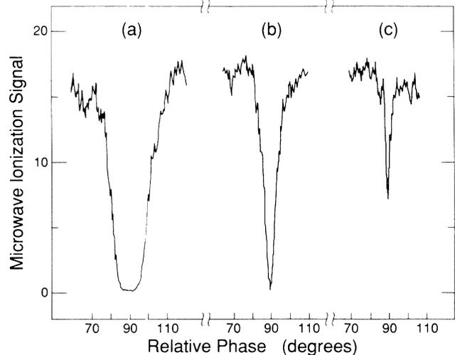
FIG. 2. Microwave ionization signal as a function of relative phase between the horizontal and vertical fields when the atoms are excited to the energy of the  $46d$  state and the attenuation is set between the linear- and circular-polarization ionization thresholds. Specifically, scans of the phase are shown for microwave fields of (a) 34.6 V/cm, (b) 53.5 V/cm, and (c) 61.5 V/cm.
