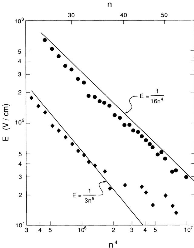
FIG. 3. Ionization threshold fields for linear (■) and circular (●) polarization as a function of  $n$  when the atoms are excited in the microwave field.
