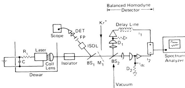
FIG. 1. Experimental arrangement and apparatus, described in detail in the text. The beam from a cryogenic GaAs laser is collimated, can be mode analyzed by a Fabry-Perot interferometer (FP), and its amplitude noise is compared with the vacuum level using a balanced homodyne detector. The movable mirror  $M_1$  is inserted for  $\text{Kr}^+$ -beam calibration of the SQL.
