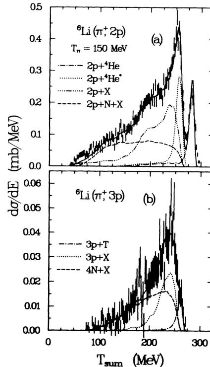
FIG. 1. (a) Summed charged-particle energy spectrum for events in which two energetic protons ( $T_p > 18$  MeV) were detected following  $\pi^+$  absorption with  ${}^6\text{Li}$  at  $T_\pi = 150$  MeV. (b) Summed charged-particle energy spectrum for events in which three energetic protons ( $T_p > 18$  MeV) were detected following  $\pi^+$  absorption with  ${}^6\text{Li}$  at  $T_\pi = 150$  MeV.
