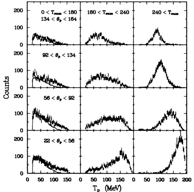
FIG. 2. Histograms of the energy distributions of protons from two-proton events with different cuts on the summed energy  $T_{\text{sum}}$  (columns), and for different scattering angles  $\theta_p$  (rows). The solid lines for the column ( $0 < T_{\text{sum}} < 180$ ) are the result of  $3N+X$  normalized to the data.
