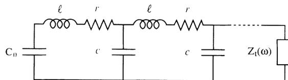
FIG. 1. A schematic model of a tunnel junction  $C_0$  connected to an  $RLC$  transmission line terminated by an impedance  $Z_l(\omega)$  after a length  $d$ .
