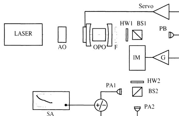
FIG. 1. Experimental setup. AO: acousto-optic modulator; F: dichroic filter; HW1, HW2: half-wave plates; BS1, BS2: polarizing beam splitters; IM: intensity modulator; PA1, PA2, PB: photodetectors; SA: spectrum analyzer.
