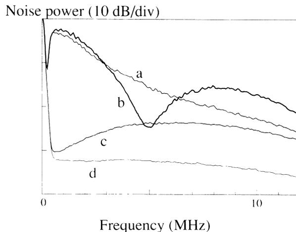
FIG. 2. Experimental noise spectra of beam *A* (curve *a*) without feedforward correction, (curve *b*) with feedforward correction, (curve *c*) associated shot-noise level, and (curve *d*) electronic noise.
