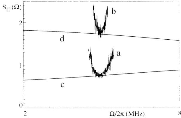
FIG. 3. Experimental noise spectra of beam *A*, normalized to the shot-noise level, (curve *a*) when the two beams at the OPO output are quantum correlated and (curve *b*) decorrelated by the beam mixer HW1+BS1. The largest noise power reduction is 24% below the shot-noise level (curve *a*). Theoretical curves (*c* and *d*) represent the minimum obtainable noise powers for these cases when the gain is optimized at every frequency.
