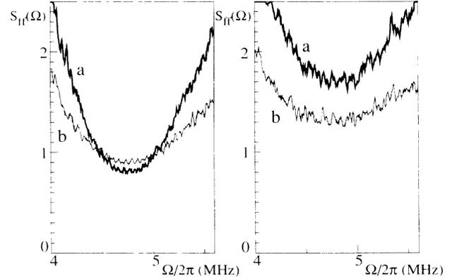
FIG. 4. Effect of a 50% attenuator inserted in beam *A* after the intensity modulator, (left) when the two beams at the OPO output are quantum correlated and (right) decorrelated. Curves *a* are the noise spectra of beam *A* without attenuation, while curves *b* are the noise spectra with attenuation. As expected, the attenuated noise tends toward the shot-noise level in proportion to the amount of attenuation.
